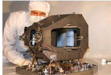
JWST NIRSpec instrument optics [early universe search]
